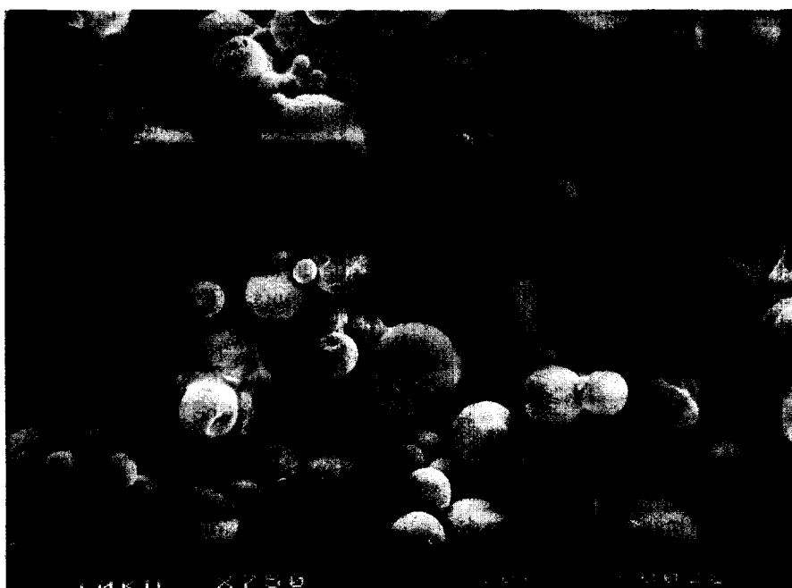
Fig. 1. SEM photomicrograph of spray-dried lactose particles, stored at 0% RH after spray-drying.
